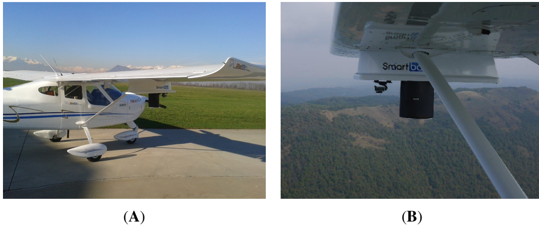
Figure 8. Sensor prototype mounted on the manned Digisky Tecnam P92 aircraft ready to take off (A) and during the flight (B).
