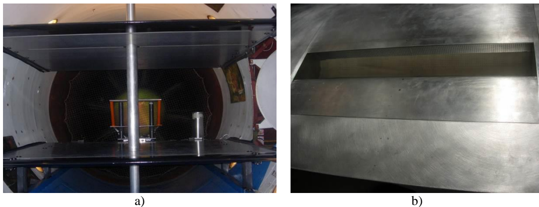
Fig. 3 - The wing model and the module with the trapped vortex cell.
