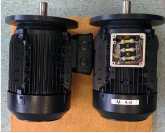
Figure 8: Induction Motors for the experimental tests.
