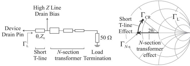
Fig. 2. Proposed OMN and implemented matching trajectories.
