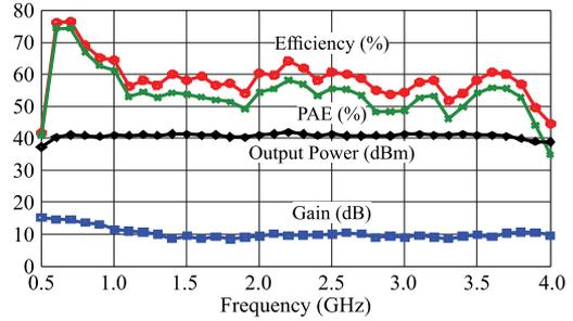
Fig. 8. Measured saturated gain, saturated output power, efficiency and PAE (at saturation) vs. frequency.
