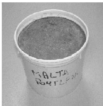
Fig. 11. Sample cured at constant humidity after five years of its preparation (Portland Job site, USA – photos Mapei's archive).
