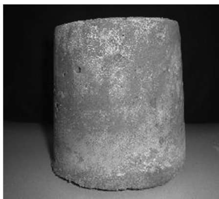
Fig. 11. Sample cured at constant humidity after five years of its preparation (Portland Job site, USA – photos Mapei's archive).
