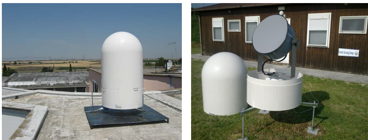
Figure 1. Short range X-band single polarization mini weather radar with high temporal and spatial resolution.
