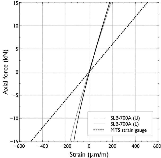
**Figure 9:** Strain measured in cyclic axial loading tests on a 30 mm × 5 mm steel bar. SLB-700A (U) and (L) denote the positions of the instruments: upper and lower, respectively. The dashed line corresponds to the measurements obtained from the forceless transducer positioned at the midpoint of the bar.
