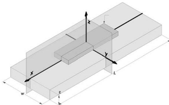
**Figure 4:** Schematic of the configuration analysed with the finite element method. Homogeneous opposite displacements in the  $x$  direction are imposed on the faces of the plate perpendicular to the  $y$  axis. Thanks to symmetry, only one quarter of the domain ( $x > 0$ ,  $y > 0$ ) has been discretized.
