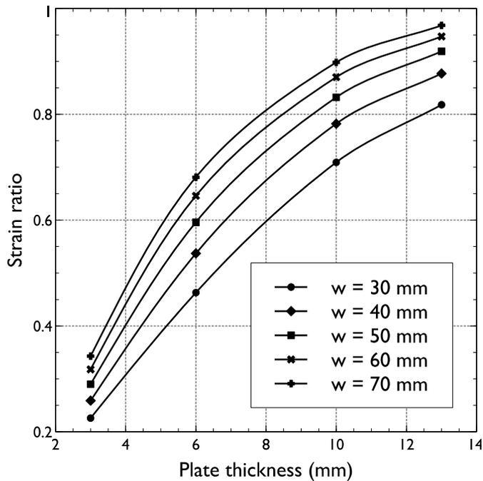
**Figure 7:** Synthesis of the results of the FEM calculations. Ratio between the strain of the transducer and the imposed strain vs. the thickness  $t$  of the plate, for different values of the width  $w$ .
