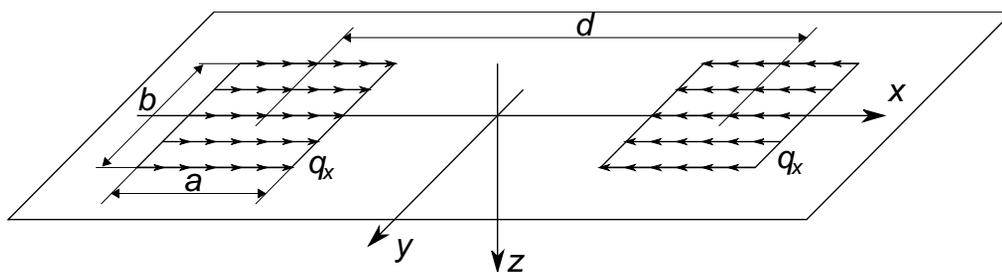
**Figure 2:** Distributions of opposite tractions  $q_x$  to evaluate the strain perturbation induced by the deformation transducer on the half-space surface. The distance between the centres of the loaded rectangles is  $d$ . The length and width of the surfaces are denoted by  $a$  and  $b$ , respectively.
