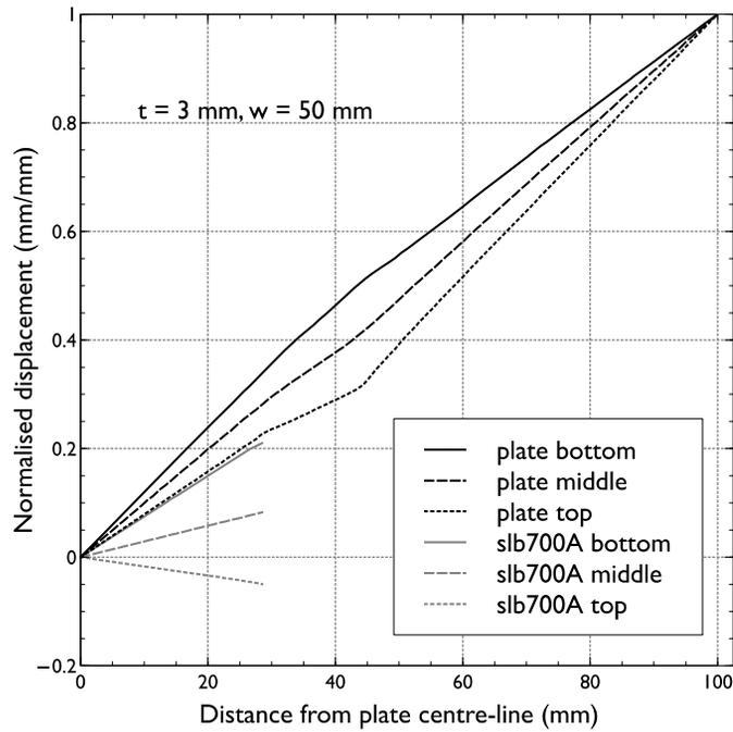
**Figure 6:** Example of the results of the FEM calculations. Axial displacements along the  $x$  axis vs. distance from the centre for  $t = 3$  mm and  $w = 50$  mm, normalized with respect to the maximum. The curves represent the displacement of points of the  $y = 0$  plane along lines parallel to the  $x$  axis at different  $z$  heights.
