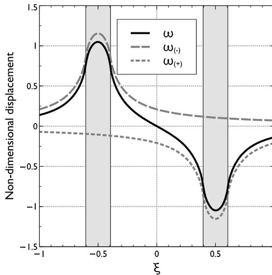
**Figure 11:** Non-dimensional displacements along the  $\xi$  axis for the SLB-700A transducer geometry. The shaded zones, centred at  $\xi = \pm 1$ , represent the positions of the loaded rectangles. The two grey lines show the separate effects of the loads; the black one is the combined result.
