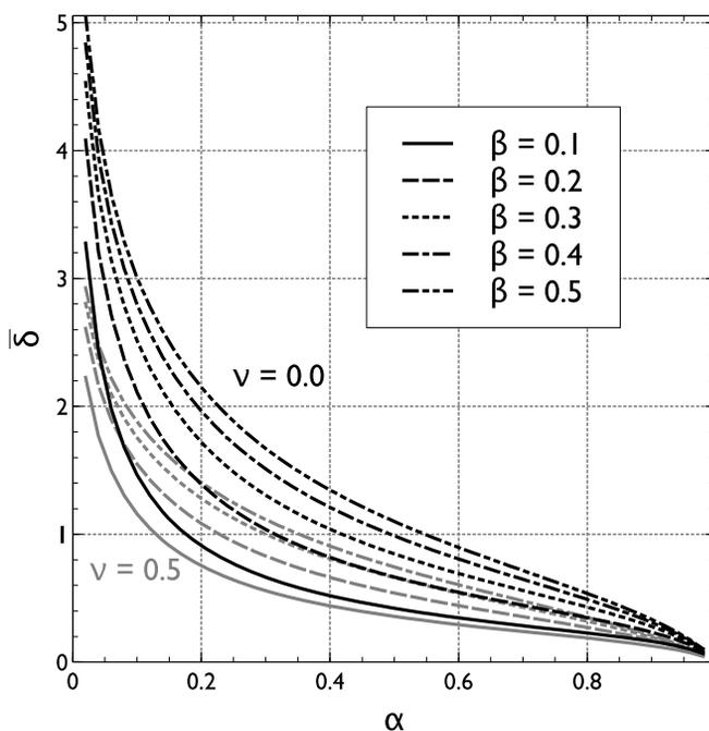
**Figure 3:** Plots of the non-dimensional relative displacement  $\bar{\delta} = 2\bar{w}$  vs. the non-dimensional length  $\alpha$  for different values of the non-dimensional width  $\beta$  of the loaded zones, and for two Poisson ratio values, namely,  $\nu = 0.0$  (black curves) and  $\nu = 0.5$  (grey curves).
