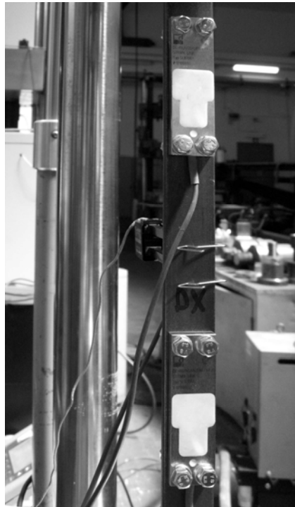
Figure 5: Setup for the SLB-700A comparison tests. The bar is placed vertically between the loading machine grips. The upper and lower transducers are clearly visible. The forceless MTS extensometer can also be seen on the other side at the midpoint of the bar.
