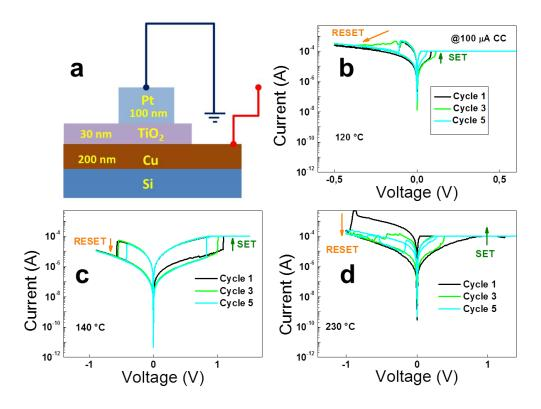
FIG. 28. Schematic diagram of the Cu/TiO<sub>2</sub>/Pt devices (a) semi-logarithmic I-V curves of devices with TiO<sub>2</sub> grown at 120 (b), 140 (c) and 230°C (d), showing the first 5 memristive cycles. The devices work in bipolar resistive switching.
