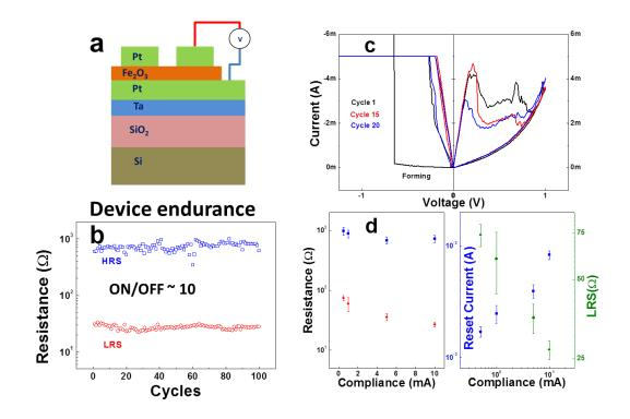
FIG. 33. Device diagram (a), cyclic I-V characteristics (b), switching endurance (c) and resistance states vs compliance current plot of Fe<sub>2</sub>O<sub>3</sub> device.
