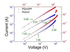
FIG. 21. Line fitting in log-log scale IV characteristics of pure and polymer-coated ZnO NW memristive devices with Pt TE.
