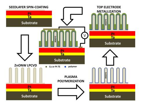
FIG. 6. Fabrication procedure for Pt/ZnO NW/Pt memristive devices.
