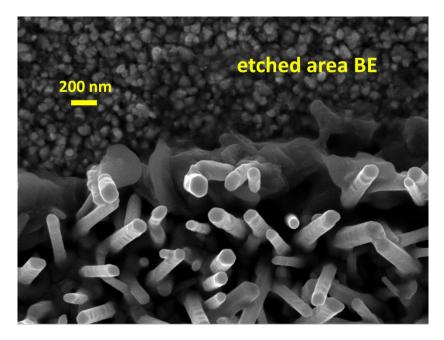
FIG. 7. FESEM of ZnO NW array showing the etched area exposing the bottom electrode.
