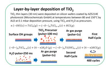
Fig. 24. Typical surface reactions during one ALD cycle of TiCl<sub>4</sub> and H<sub>2</sub>O pulsing.
