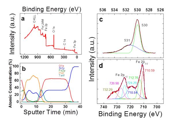
FIG. 32. XPS spectra of  $Fe_2O_3$  thin films: survey spectrum (a), depth profile (b) and high resolution spectra of O1s (c) and Fe2p (d).
