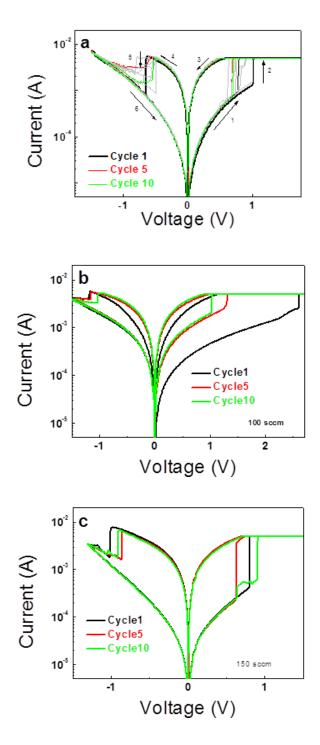
FIG. 13. A series of DC sweep plotted in semi-logarithmic IV shows the bipolar resistive switching characteristics of Pt/ZnO NW/Pt devices with different  $O_2$  flow rates: 50 sccm (a), 100 sccm (b) and 150 sccm (c).
