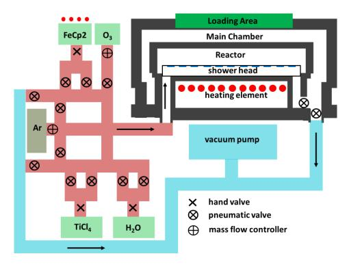
FIG. 5. Schematic diagram of the ALD reactor used for the deposition of  $TiO_2$  thin films.
