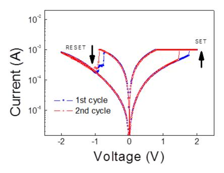
FIG. 19. The bipolar resistive switching characteristics of Cu/ZnO NW/Pt device plotted in semi-logarithmic scale.
