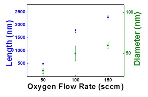
FIG. 12. ZnO NW dimensions (length and diameter) with different oxygen flow rates.
