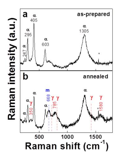
FIG. 31. Raman spectra of as-prepared (a) and annealed (b)  $Fe_2O_3$  thin films deposited by 400 ALD cycles.
