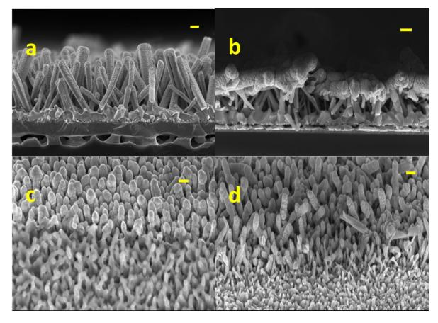
FIG. 9. FESEM of ZnO NW memristive devices: Pt/ZnO NW/Pt (a), Pt/ZnO NW/PP/Pt (b), Cu/ZnO NW/Pt (c) and Cu/ZnO NW/PP/Pt (d). scale bar = 200 nm
