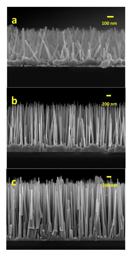
FIG. 11. Cross-section image of ZnO NWs grown with 50 sccm (a), 100 sccm (b) and 150 sccm (c)  $O_2$  flow rates.
