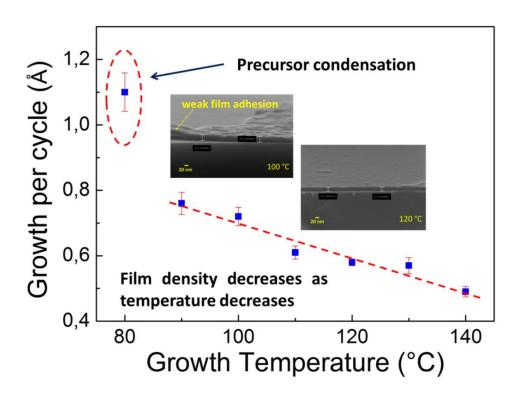
FIG. 26. Growth rate of TiO<sub>2</sub> films shows decreasing trend as temperature increases.
