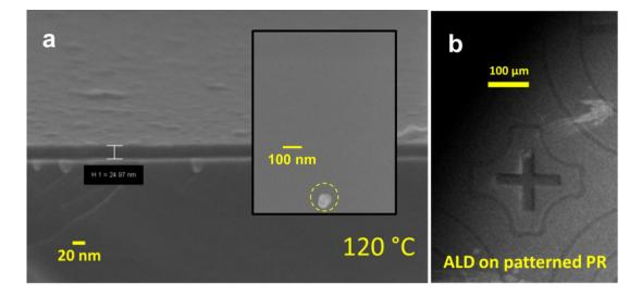
FIG. 25. FESEM image of ALD  $TiO_2$  thin film on Si substrate deposited at 120 °C (a) and effective DMSO liftoff of ALD  $TiO_2$  thin films on patterned PR (b).
