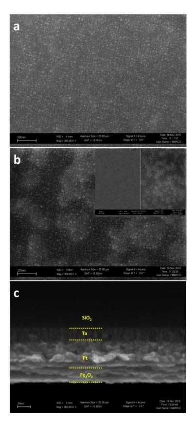
FIG. 30. SEM top view at the center (a) and edge (b) of the sample, and cross-section view (c) of  $Fe_2O_3$  thin films deposited on Pt/Ta/SiO<sub>2</sub>/Si substrate for 400 cycles.
