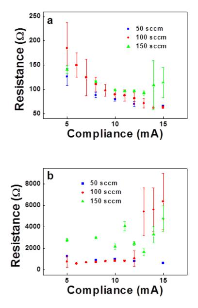
FIG. 15. Variations in devices' resistance states: LRS (a) and HRS (b) with different compliance.
