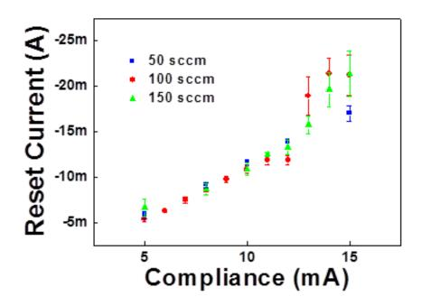
FIG. 16. Linear relation of compliance and reset current.
