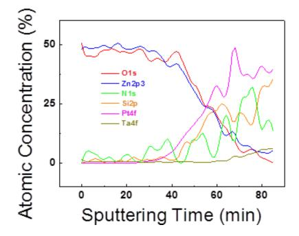
FIG. 17. XPS depth profile of ZnO NW arrays deposited on Si substrate with 150 sccm flow rate.
