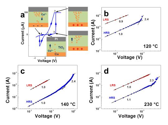
FIG. 29. Schematic diagram of the Cu/TiO<sub>2</sub>/Pt devices showing the filament formation and rupture that happens in one cycle (a) double-logarithmic I-V curves of devices with TiO<sub>2</sub> grown at 120 (b), 140 (c) and 230°C (d) showing the two resistance states.
