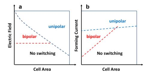
FIG. 1. Area dependence of the different switching regimes with the applied electric field (a) and forming current (b).
