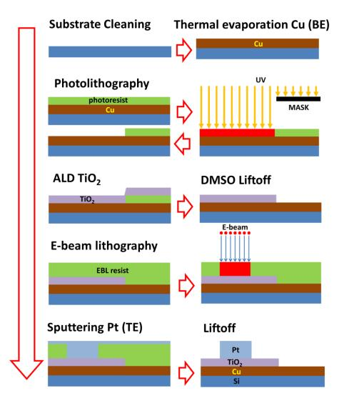
FIG. 10. Fabrication procedure for Cu/TiO2/Pt memristive devices.
