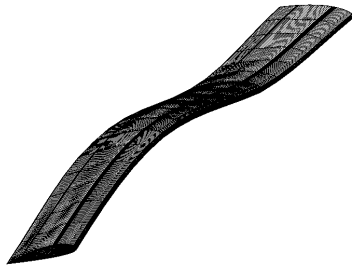
(c) Mode 5 with non-structural mass, CW model (50.47 Hz)
