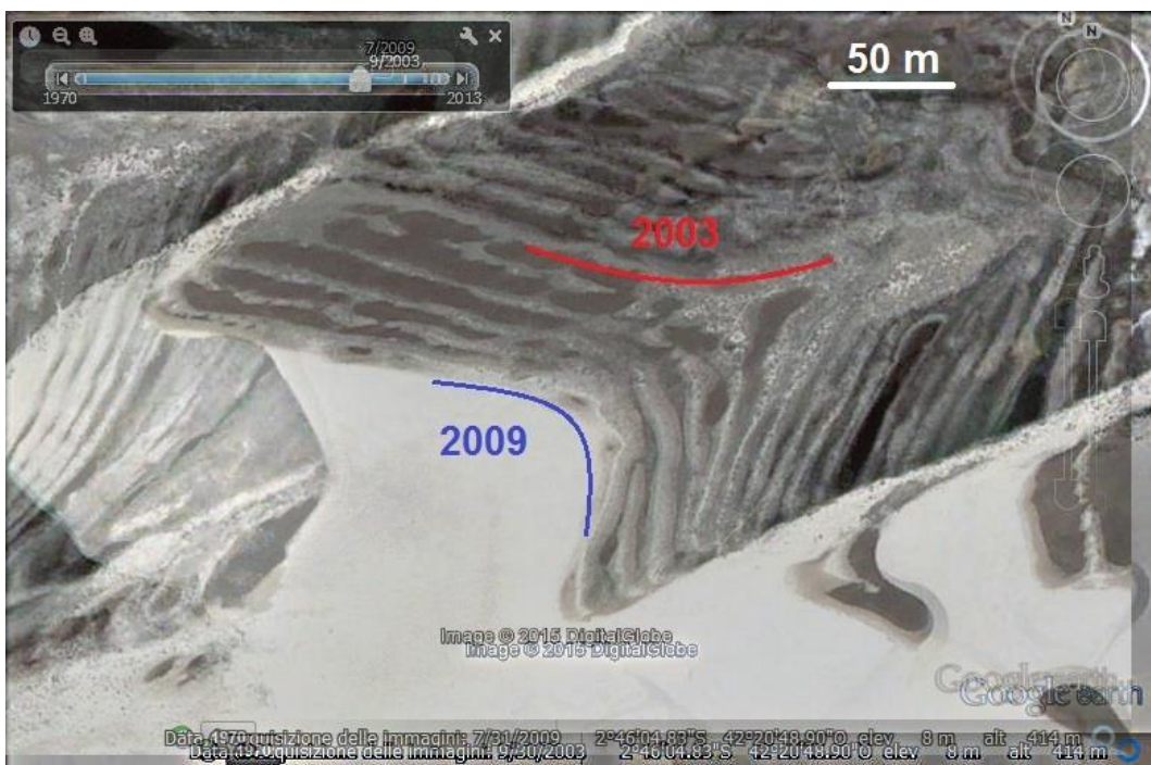
Figure 10: Also for this figure, we used GIMP to create an image from two layers adjusted with Retinex filtering. Red line marks the position of the toe of the dune in 2003, whereas blue line marks its position in 2009. The shortest distance between the red and the blue line is of 60 m.
