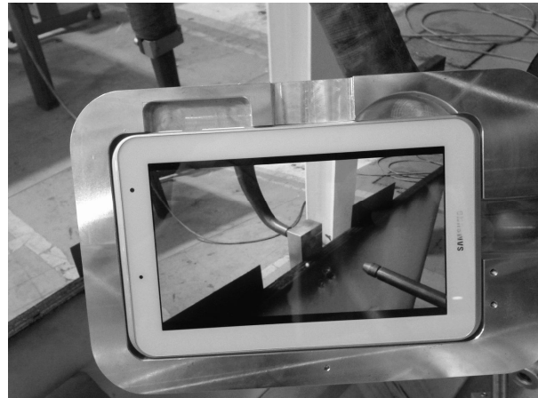
Fig. 3. The tablet mounted on the welding gun, with its built in rear camera used for displaying the real view of the clamps (maximum opening position).
