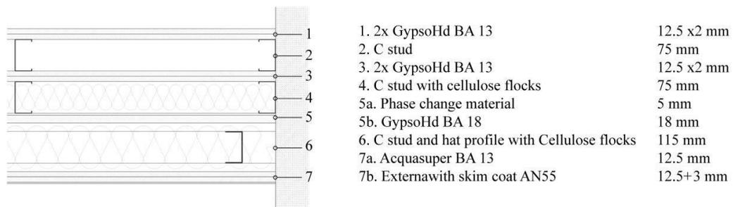
Figure 1. Wall cross section of the INTESA system.
