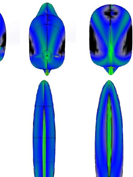
The selected design solution resulted competitive with these reference prototypes in terms of drag and, as a consequence, in terms of power required to travel at a given speed. Also lift forces were compared showing a reduced down-force for PulsaR, lowering the effect of tire load increase with speed and resulting in less overall rolling resistance.
