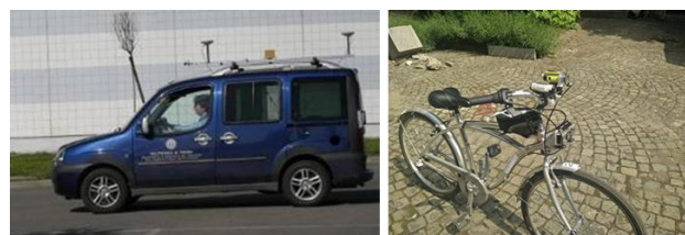
Figure 2. Mobile Mapping System on car and bicycle
