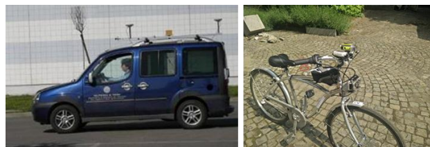
Figure 2. Mobile Mapping System on car and bicycle
