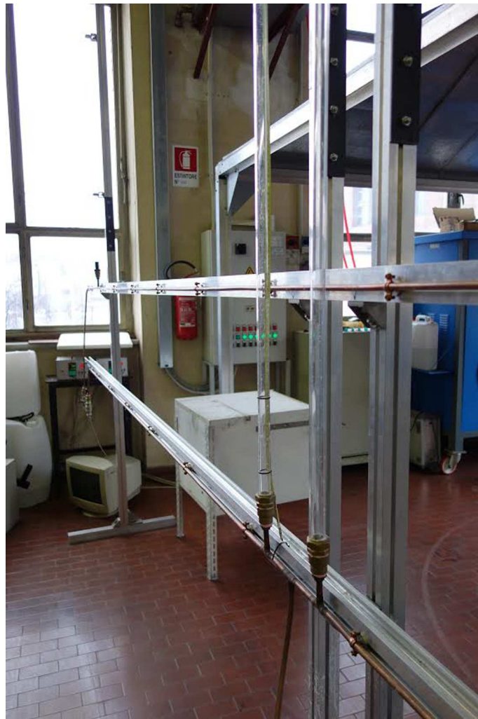
Figure 4 Experimental setup for pressure drops determination.
