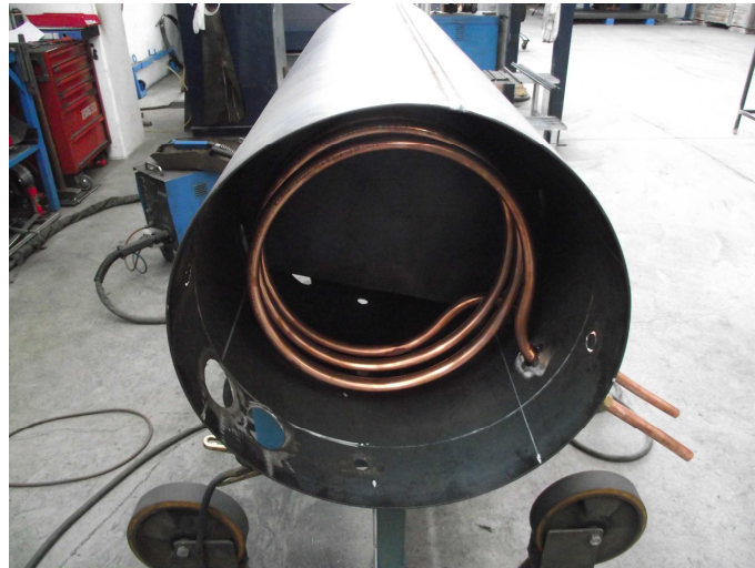
Figure 6 View of the interior of the storage tank and the heat exchanger.
