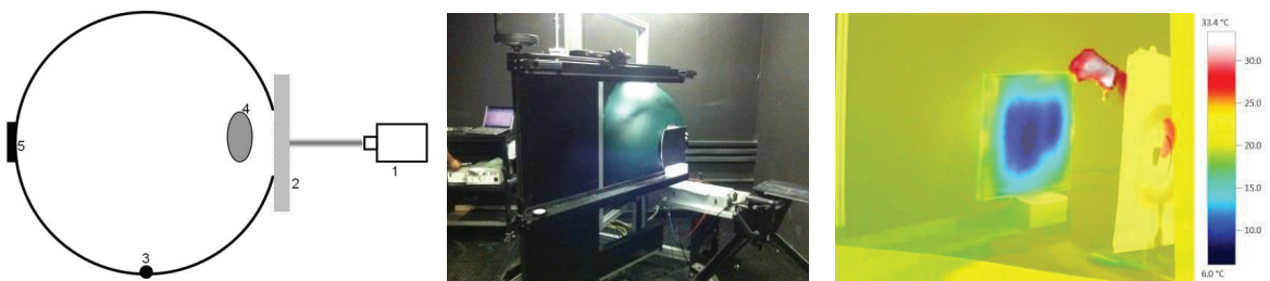
Figure 2. Optical bench apparatus in transmittance modes (left). Main parts: 1-light source; 2-sample port (transmittance port) with holder; 3-opticfibre connected to the detection system; 4-auxiliary port; 5-reflectance port. Optical bench in reflectance mode (middle). Infrared thermal image of the sample A during the measurement (right)
