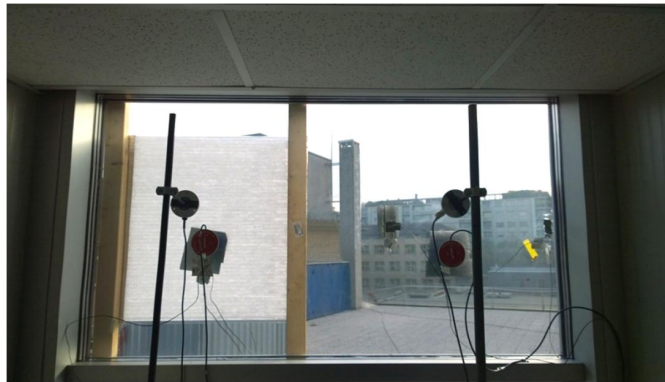
Fig. 2 An internal view of the test cell with the PCM shutter
