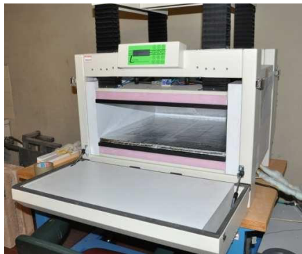
Fig. 1. Guarded heat flow meter apparatus.
