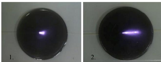
**Figure 4.** Example of two delivery fibres with different radiation pattern: a normal (left) versus a surface modified fibre (right). In both cases the fibres are inserted into an agar phantom with the temperature sensing FBG fibre in close proximity.
