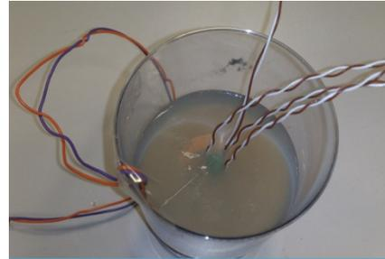
**Figure 2.** Liver phantom with resistor and thermocouples
