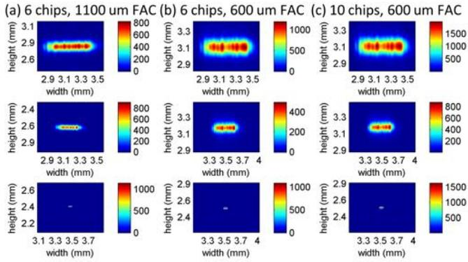
**Fig. 14.** Visual comparison of the impact of the focusing lens for the combination beams using different FACs and 12 000  $\mu\text{m}$  SAC. The first row is for a focusing lens with EFL = 100.1 mm, the second for a lens with EFL = 49.8 mm and the third for a lens with EFL = 8 mm.
