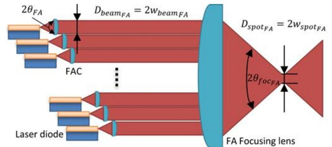
**Fig. 4.**  $N_{\text{FA}}$  laser diodes arrangement along the FA; besides for the vertical stacking, the picture shows also a longitudinal offset, which is necessary for the practical implementation of the multi-emitters but does not impact on the model derivation.
