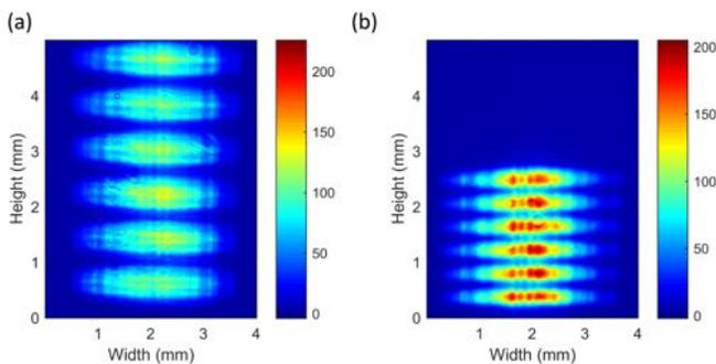
**Fig. 12.** Comparison of the images at the entrance of the focusing lens for the combination of 6 chips: (a) 1100  $\mu\text{m}$  FAC, and (b) 600  $\mu\text{m}$  FAC.
