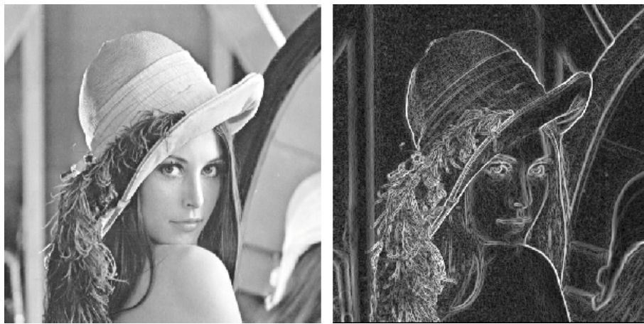
Fig.1 The original image on the left. On the right, the map obtained evaluating the magnitude of local dipole moments, according to Eqs.10 and 11. Note that this map is giving the image edges.
