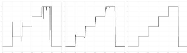
Figure 11 - Failure detection output for different types of failure, original detection logic output at the left. Errors in the detection are caused by instantaneous equivalence between the failed output state and the commanded one. As these errors are usually one sample long, they can be easily filtered out.
