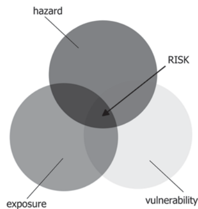
Figure 20.2: Risk considered as the superimposition of three constitutive factors, H (hazard), E (exposure), V (vulnerability) (Franzi, 2012).
