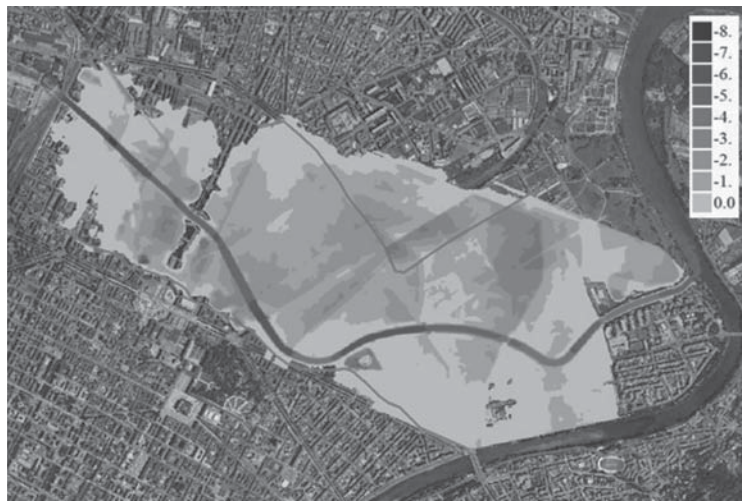
Figure 20.9: Inundation map due to Dora Riparia Q_{500} flooding. The depths are expressed in meters (Bruno 2013).
