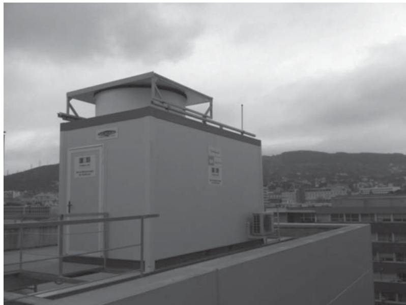
Figure 18.3: Automatic Radiosounding Station located on the roof of the Faculty of Physics (University of Barcelona).
