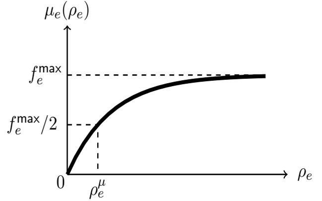
Fig. 3. Qualitative behavior of a flow function satisfying Assumption 2:  $\mu_e(\rho_e)$  is differentiable, strictly increasing, has bounded derivative and such that  $\mu_e(0) = 0$ , and  $\lim_{\rho_e \rightarrow \infty} \mu_e(\rho_e) = f_e^{\max} < \infty$ . The median density  $\rho_e^\mu$ , as defined in (5) is plotted as well.
