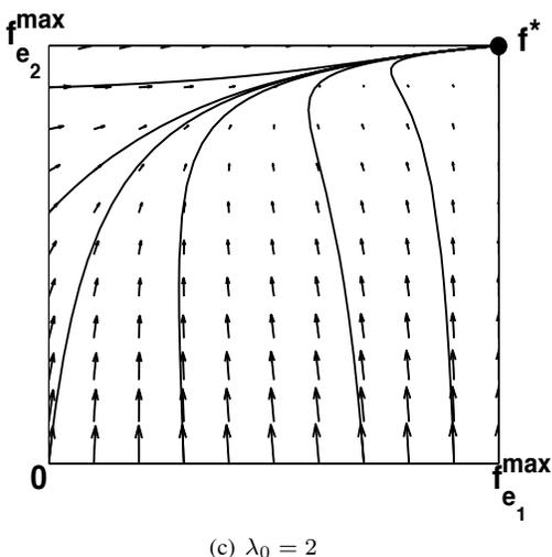
Fig. 6. Flow vector fields and flow trajectories for the dynamical network of Example 4, for three values of the inflow. In the first two cases  $\lambda_0 < \lambda_0^{\max}$ , and hence the limit flow  $f^*$  is an equilibrium flow. In contrast, in the last case,  $\lambda_0 \geq \lambda_0^{\max}$ , and consequently  $f^*$  is not an equilibrium flow and  $f_{e_1}^* = f_{e_1}^{\max}$  and  $f_{e_2}^* = f_{e_2}^{\max}$ , as predicted by Theorem 1.
