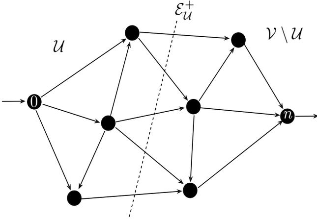
Fig. 2. An origin/destination cut of the network:  $\mathcal{U}$  is a subset of nodes including the origin  $0$  but not the destination  $n$ , and  $\mathcal{E}_U^+$  is the subset of those links with tail node in  $\mathcal{U}$ , and head node in  $\mathcal{V} \setminus \mathcal{U}$ .
