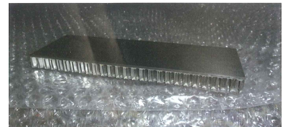
Figure 1 - Composite sandwich laminate object of the study
