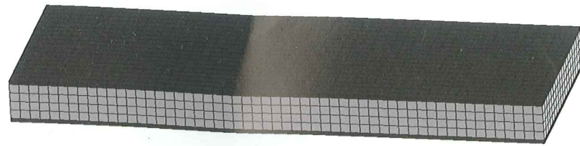
Figure 2 - Shell-brick-shell model of the sample of the sandwich laminate
