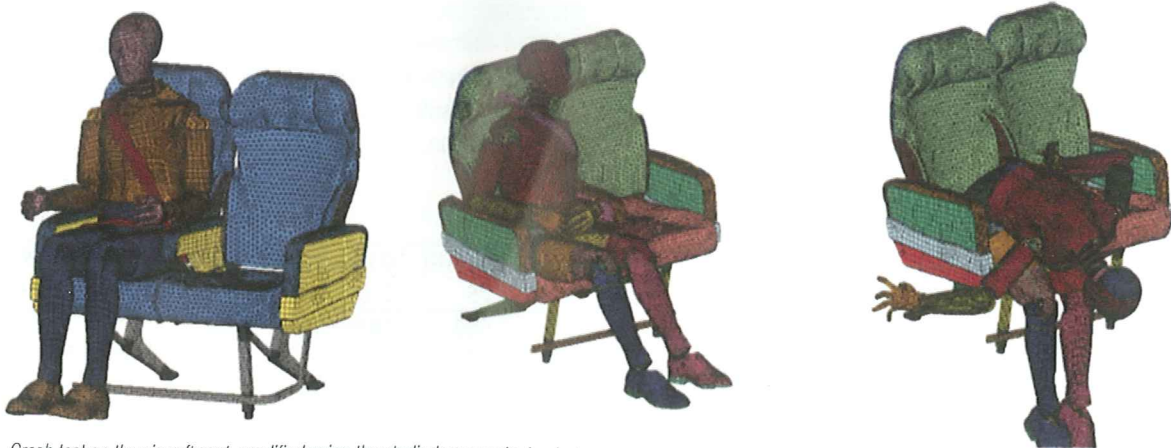
Figure 11 - Crash test on the aircraft seat, modified using the studied composite laminate
