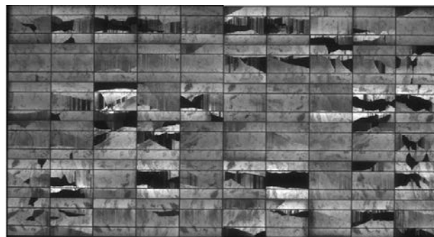
Fig. 16. EL image of a 60 p-Si cell module with high occurrence of cracks.
