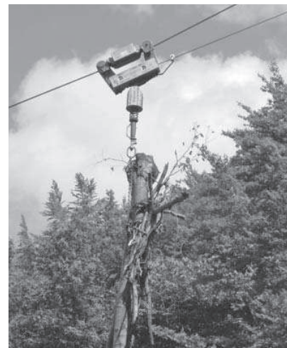
Fig. 2. Yarder's truck. Carrello della gru a cavo.
