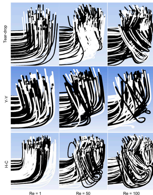
Figure 6. Path lines at the exit of the micromixers at different Reynolds numbers.
