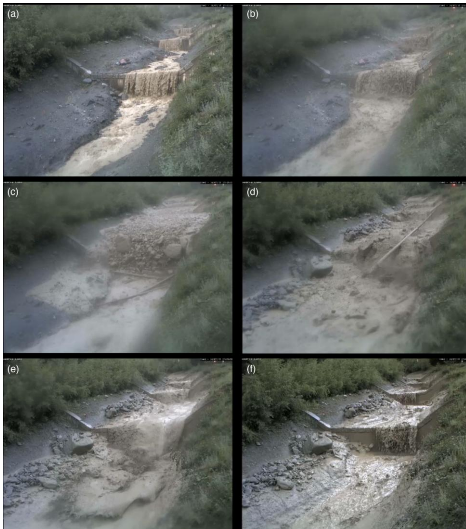
Figure 52 - Frames from the video camera of the debris flow event that occurred on July 15, 2014 in the Gatria basin. In the upper right corner of each frame is visible the flashing light. From above, from left to right: (a) the torrent before the process (light off); (b) the precursory surge arrival (light on); (c) the main front (light on); (d) and (e), two secondary surges (light on); (f) the end of the flow process (light off).
