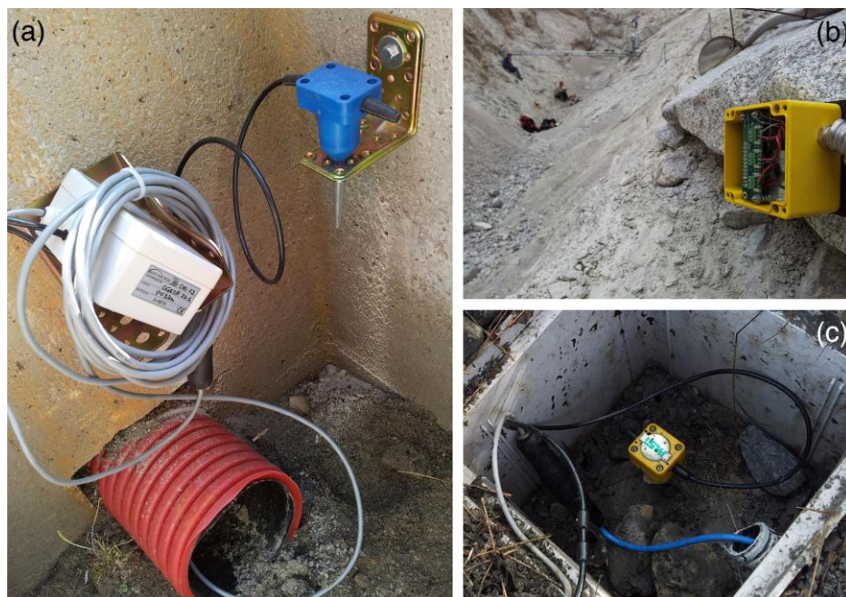
Figure 4 - Different methods of installation of the geophones: (a) embedded in a concrete manhole, picture taken in the Gatria basin (Northeastern Alps, Italy); (b) fixed on rock, Chalk Cliff monitoring station (Colorado, USA); (c) directly dug in the ground, Marderello catchment (Northwestern Alps, Italy).
