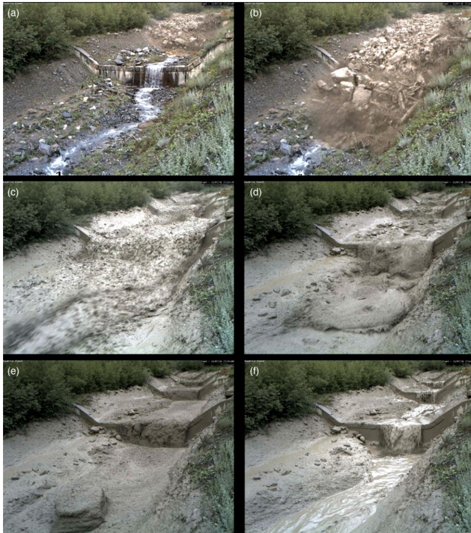
Figure 50 - Frames from the video camera recordings of July 18, 2013 at station 4. From above, from left to right: in (a) and (b), the main front arrival; in (c) and (d), two secondary surges; in (e) a late surge transporting a large boulder and in (f) the end of the flow process.
