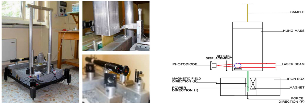
Figure 2. (a) The testing setup. (b) Micrometer slides, magnet for forced oscillation testing and hung mass. (c) He-Ne laser beam generator, attenuator and mirrors. (d) Schematic representation.
