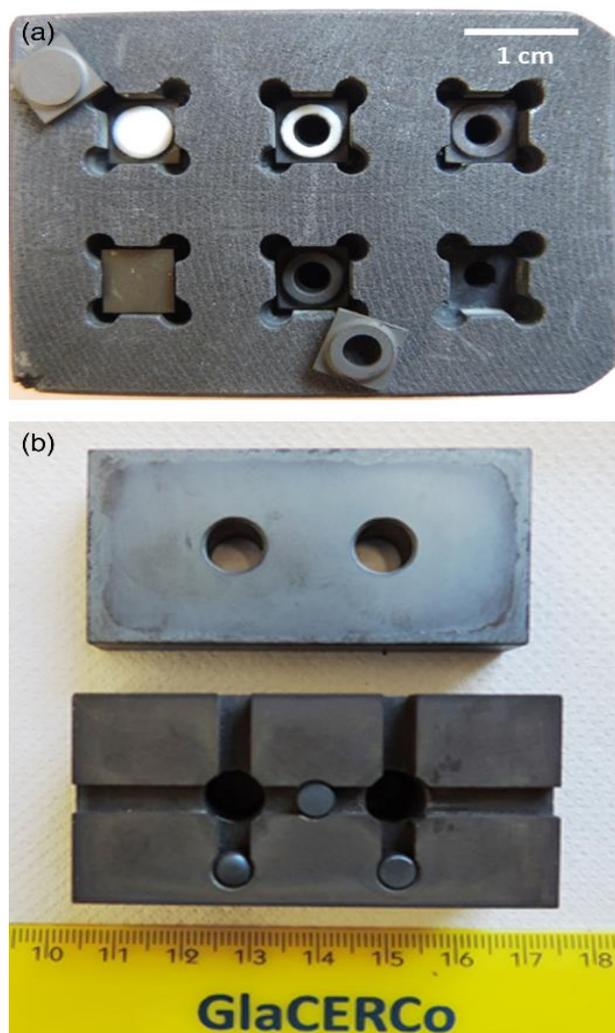
**2** a graphite sample holder with glass slurry deposited on two half hourglass samples, THG (upper part, left) and TDHG (upper part, centre) and ready to join hourglass samples (lower part) and b stainless steel sample holder for joining of ISO 13124 cross-bonded samples
