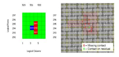
Figure 3.23: An irregular cluster showing many physical defects.
