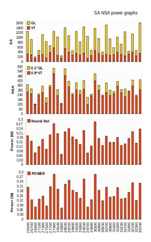
Figure 5.9: SA, NSA, FFNN power estimation and power evaluation of a sample program.
