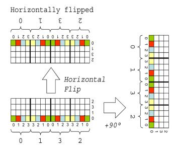
Figure 3.6: Rotated and flipped SRAM configurations
