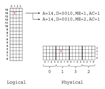
Figure 3.8: BIST responses and logical-physical fault location
