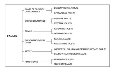
Figure 1.2: Fault classification
