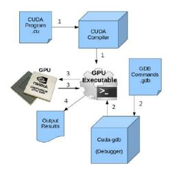
Figure 7.5: Fault Injection Environment.
