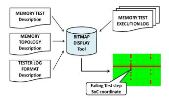
Figure 3.2: Conceptual view for Bitmap Display tool
