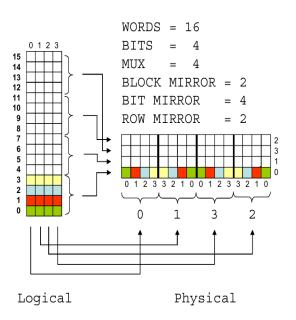
Figure 3.5: Memory logical to physical view with all mirrors
