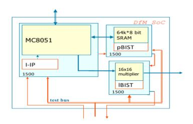
Figure 4.2: Block diagram of the test-chip
