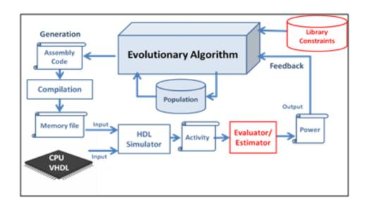
Figure 5.1: Automatic functional pattern generation framework
