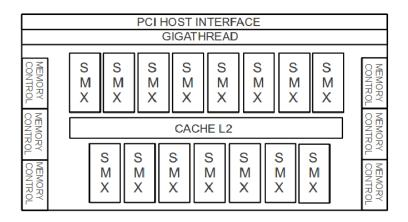
Figure 7.1: A Simplified GPGPU Architecture.
