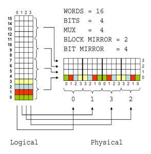
Figure 3.4: Memory view with block and bit mirrors
