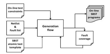
Figure 6.7: Conceptual view of the proposed generation approach
