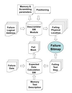
Figure 3.9: Conceptual working principle of the proposed framework
