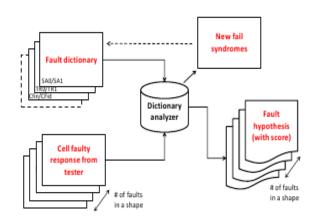
Figure 3.19: logical hypothesis produced by comparing the gathered syndrome with known fault type responses
