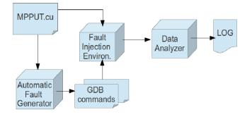
Figure 7.3: Architecture of the proposed fault injector
