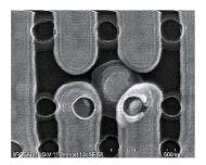
Figure 3.15: Identified defective mechanism, a stuck-open fault
