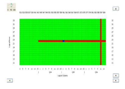
Figure 3.17: Bitmap with a partial row and a column shaped failures
