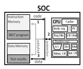
Figure 2.2: Embedded CPU under SBST testing
