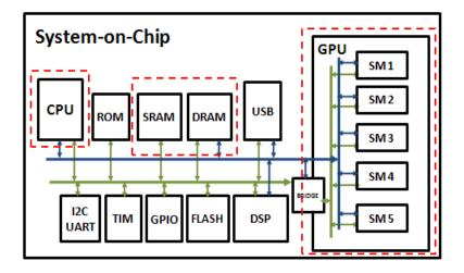
Figure 2.1: SoC Architecture
