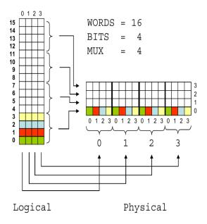
Figure 3.3: Basic mapping between logical and physical SRAM view
