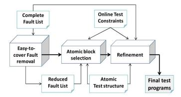
Figure 6.10: Proposed framework for on-line testing
