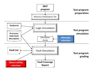
Figure 6.4: Fault Grading Environment
