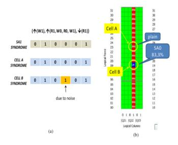
Figure 3.20: Noisy test environment affecting fault model selection: in (a) the March test executed and a comparison within expected and obtained syndromes, in (b) the shape of the failure including fault model hypothesis.
