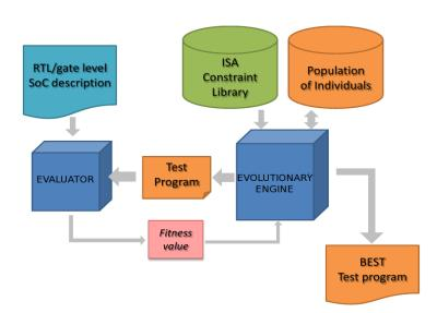
Figure 2.4: Feed-back framework for Automatic Functional Pattern Generation
