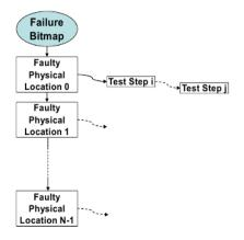
Figure 3.10: Failure bitmap data structure
