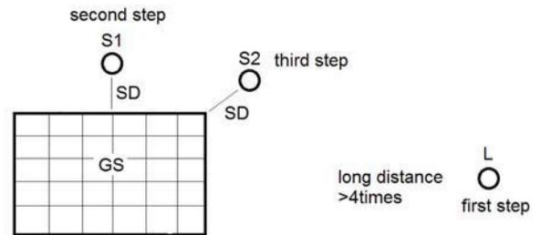
Figure 7 Locations of a sole probe at short distance
