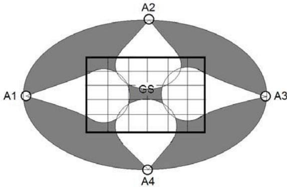
Figure 6 The gray zones are potentially the locations where the error can influence the results of  $U_t, s$  in a not conservative way.
