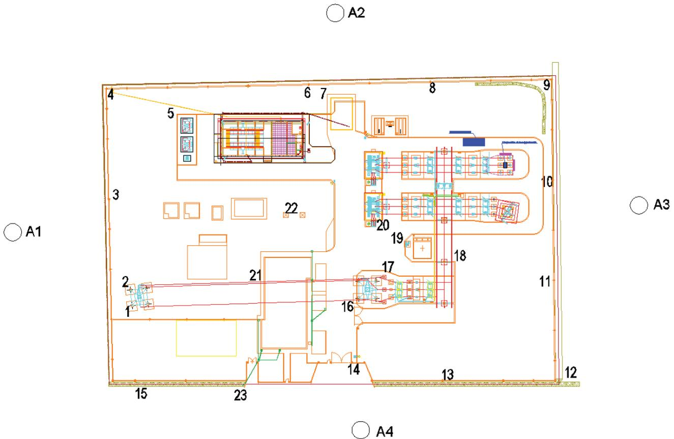
Figure 10 Grounding system of a HV/MV substation situated in Carpi (Italy): tested points
