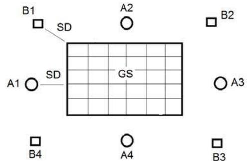
Figure 8 Locations of more probes at short distance
