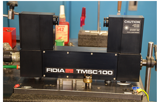
Fig. 5. The Fidia's TMS tool.
