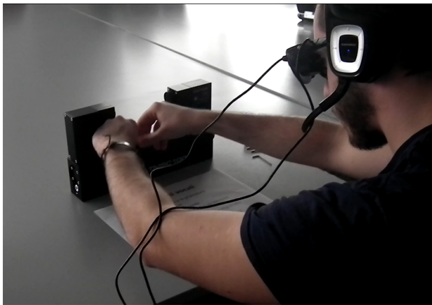
Fig. 7. A student technician performing the training procedure on the TMS tool by the AR-glasses client.
