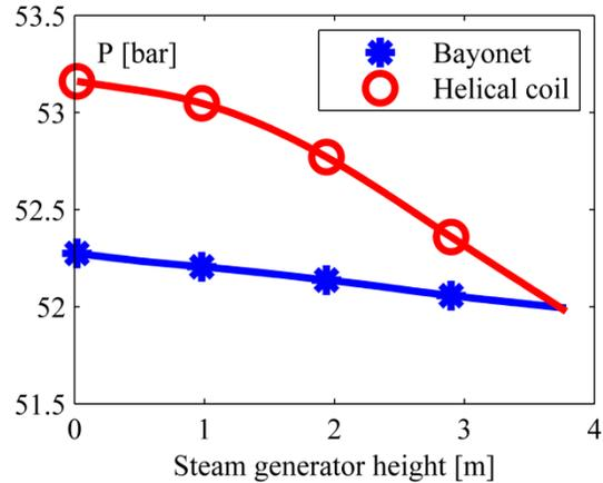
Fig. 3. Pressure profile in the secondary fluid.
