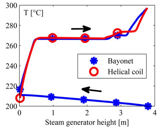
Fig. 4. Temperature profile in the secondary fluid.
