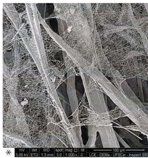
Fig. 2 - NC13 media, showing nanofiber web applied to upstream face of cellulose support media (1000x)
