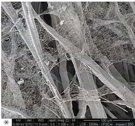
Fig. 1 Nanofiber/cellulosic media, 1000x.
