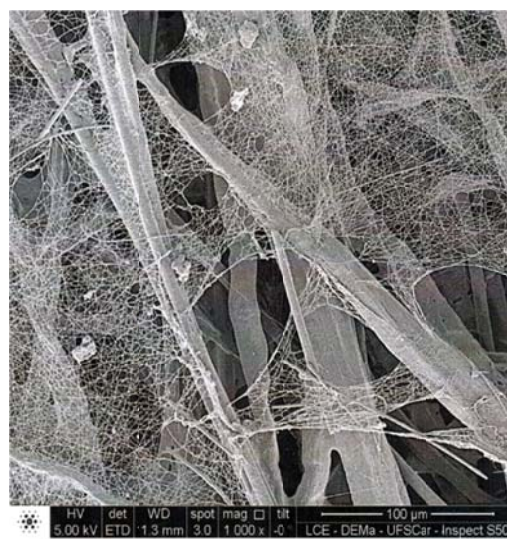
Fig. 2 - NC13 media, showing nanofiber web applied to upstream face of cellulosic support media (1000x)
