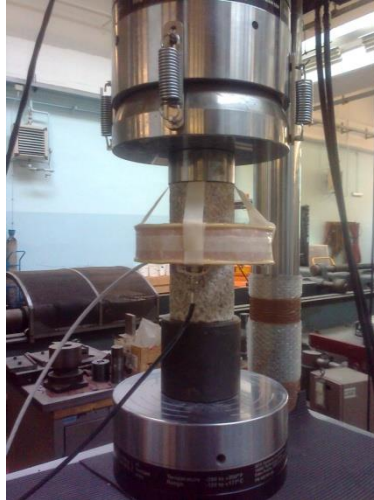
Figure 4.2: AE piezoelectric transducer positioned around the monitored gypsum specimen.
