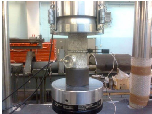
Figure 3.29: Experimental set up of the compression test on a cylindrical concrete specimen.
