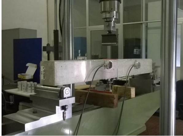
Figure 3.11: Experimental set up of the three point bending test.
