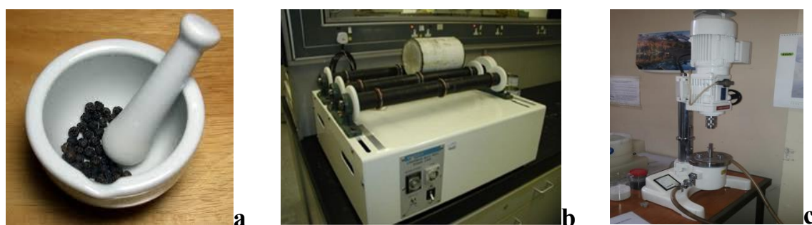
Figure 3.3 Milling of carbonized particles via mortar and pestle (a), ball milling (b) and attrition milling (c)
