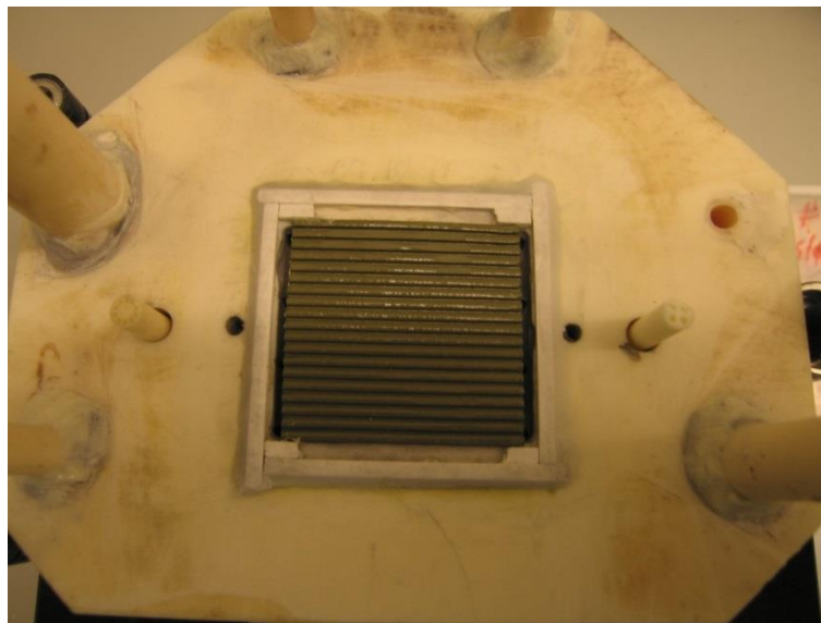
Figure 19: fuel housing with flow field distribution
