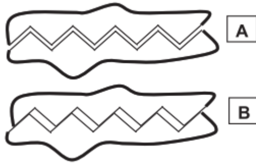
Figure 1.4: Model of a rough crack interface, (a) open crack, (b) slip at contact surfaces (Mróz & Mróz, 2010)
