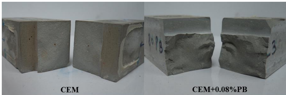
Figure 1.39: Typical fracture surfaces of the cement paste after third-point bending test
