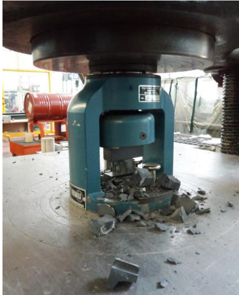
Figure 1.19: Compression test setup of cement paste composites
