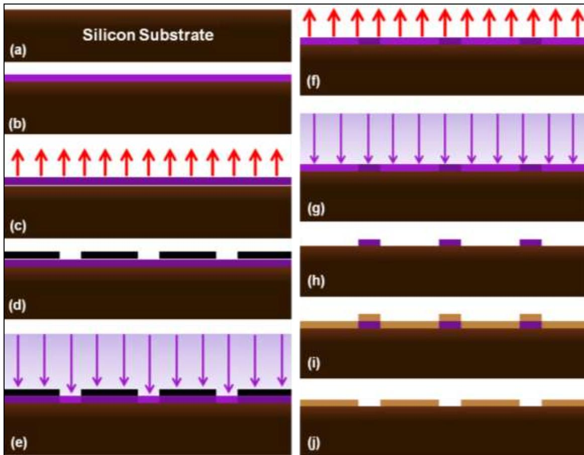
**Figure 9 Steps involved in transferring of mask to the substrate in image reversal mode a). Cleaning of wafer, b). Uniform application of photoresist by spin coating, c). Soft baking at 120°C, d). In contact mask alignment on photoresist surface, e). Controlled UV exposure, f). Reversal Bake at 120°C, g). Flood exposure, h). Development of structures, i). Metallic deposition by electron beam deposition, j). Lift off process.**
