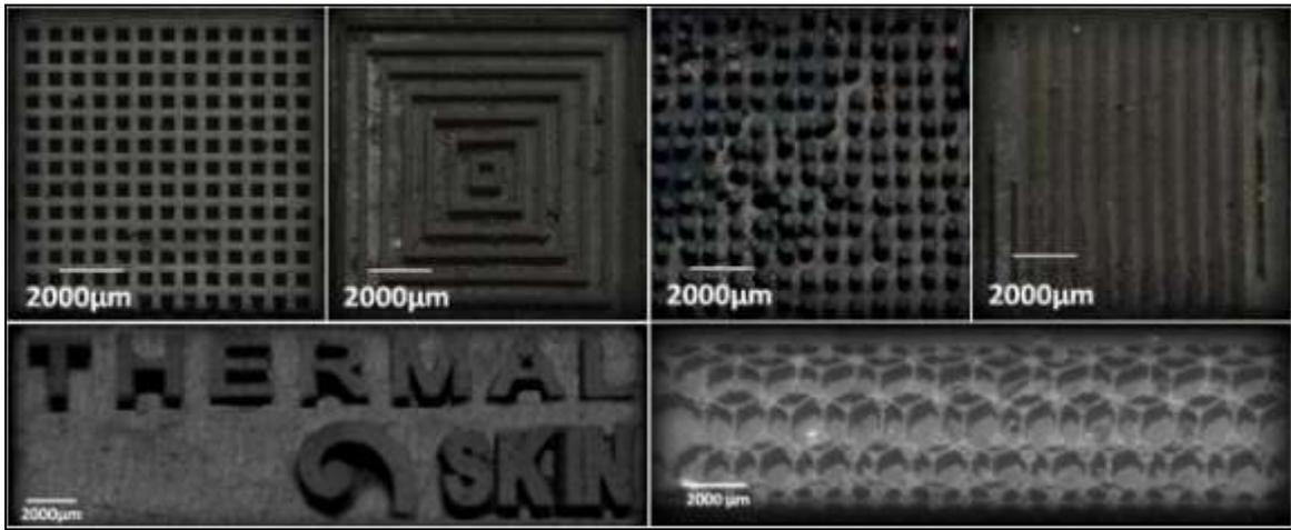
Figure 12 CNTs based structures grown by CVD Technique
