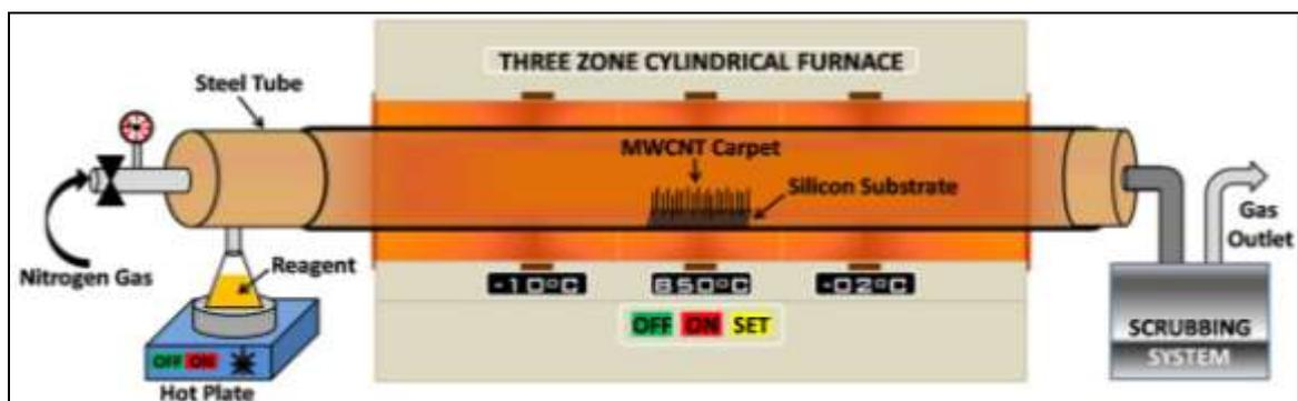
Figure 10 Thermal Chemical Vapor Deposition Growth System
