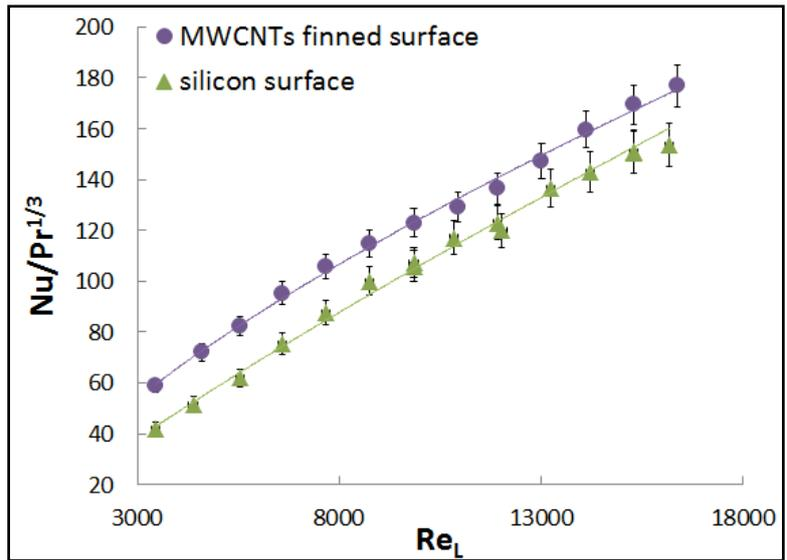
**Figure 16 Dimensionless heat transfer coefficient values in heat transfer coefficient of MWCNTs finned surface with regard to bare silicon one. All data are reported versus the Reynolds number. For MWCNTs finned surface and silicon surface (in Eq. (1)  $A = 1.123 \times 10^{-4} \text{ m}^2$  is the base area for all samples).**
