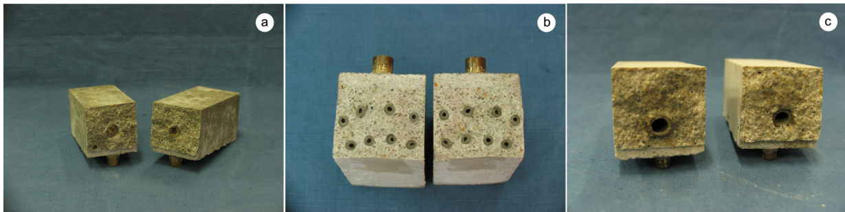
Figure 3. Mortar prisms used for the evaluation of the effectiveness of the proposed self-healing system at the end of 3-point-bending tests: (a) sample containing one big hollow tube filled with sand grains (MI series); (b) sample with 4 bucatini in the lower portion and 4 additional bucatini in a central position (BU series); (c) sample with only 1 maccherone (MS series).
