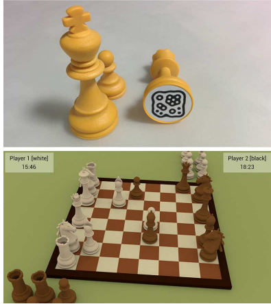
Fig. 5. A chess game developed with GAINÉ: the playing pieces and their associated fiducials (up) and a snapshot of the game view displayed on the secondary screen (down).
