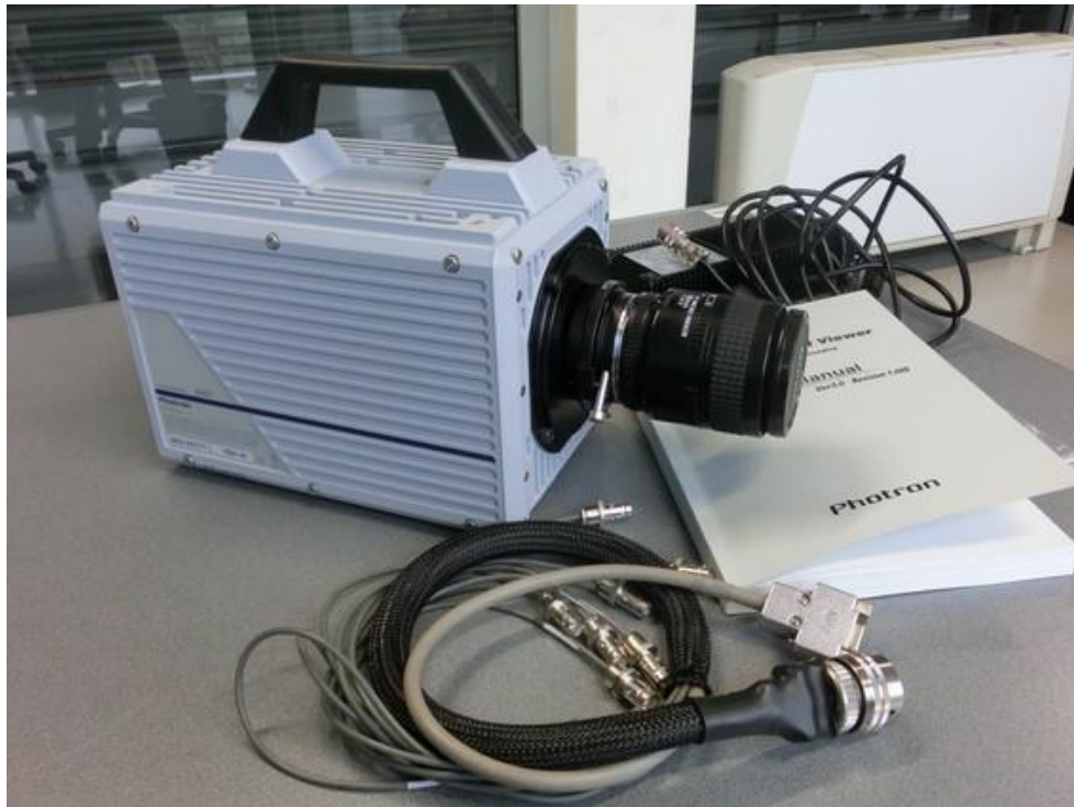
Fig. 3.14: High speed camera Photron Fastcam SA5.
