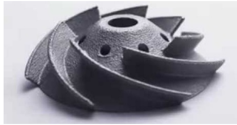
Figure 3.3: An example of a TiAl intermetallic turbine component by EBM [22]
