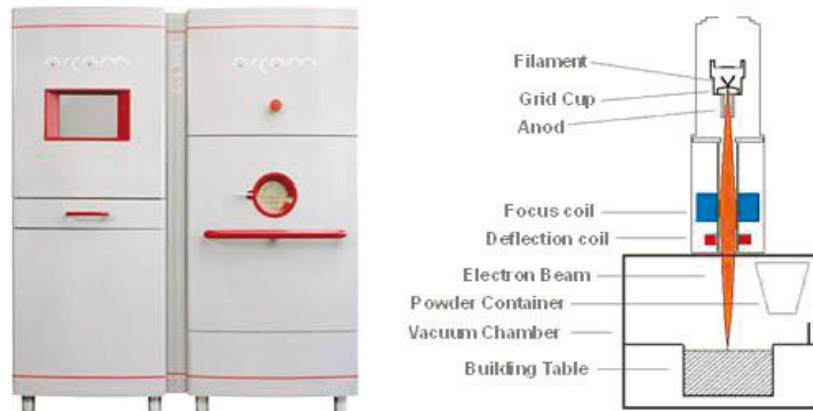
Figure 3.4: Electron beam melting, EBM: System A2 ARCAM (Sweden) on the left, and EBM process scheme, right [23]
