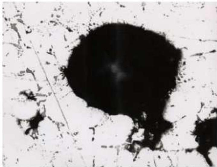
**Figure 11:** Gas porosity (courtesy of Teksid Aluminum).
