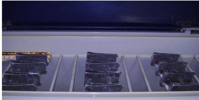
**Figure 59:** Position of the samples inside the batch during salt spray corrosion test.
