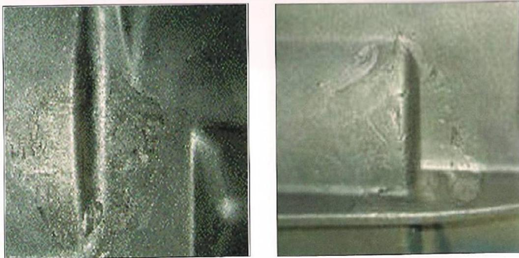
**Figure 18:** Cold shut revealed in some aluminum components [19].
