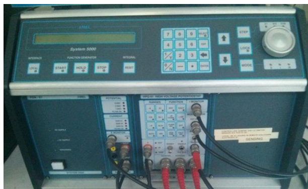
Figure 0.13 AMEL 5000 Potentiostat/Galvanostat, controlling the growth process.
