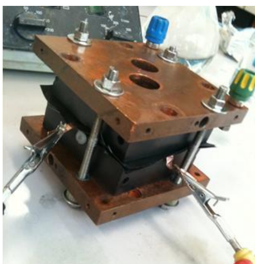
Figure 0.3 Supercapacitor test cell based on two electrodes cell configuration (actual device).
